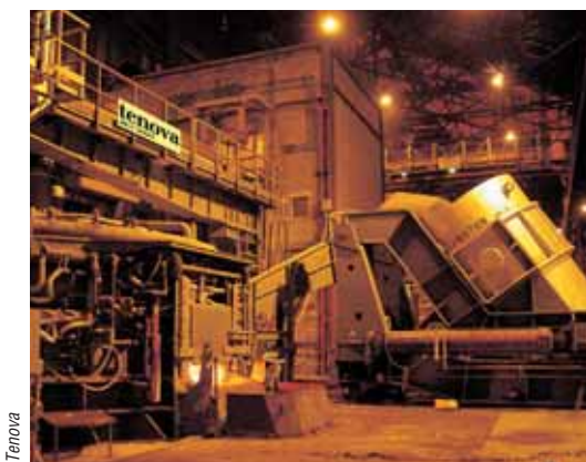
Adding hot metal to a Consteel EAF via a tilting ladle at Wheeling Pittsburgh Steel
