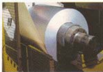
Figure 6. Strip being coiled at exit section
