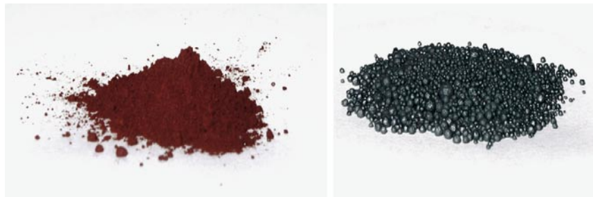
Figure 1. Powdered oxide from the spray roast process (left) and granular oxide from the fluidised bed process
