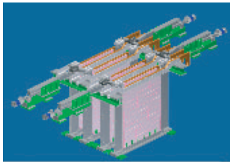
Fig 4 a &amp; b Edge masks in position in plating cells
