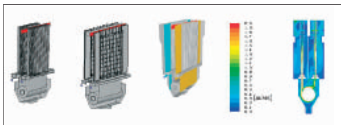
Fig 2 Plating cell configurations and speed distribution within the cell
