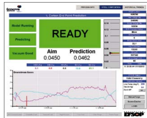
iBOF® operator screen for comprehensive process control
